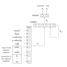
Figure 3: The architecture of the Elman network. There is one such network embedded within every voxel. We list the outputs on top and the inputs to the left: these include the vote and the actuation of the six adjacent neighboring voxels of the previous time steps.
